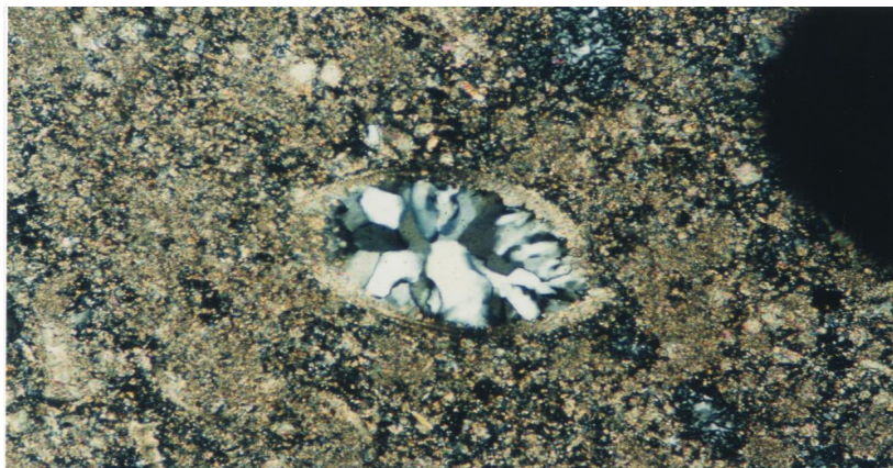
Figure 2. Photomicrograph of silty sandy limestone at East Broad Cove showing ostracode shell filled with drusy quartz cement. (sample ESS1C). Crossed polars; width of view is 2.5 mm.
